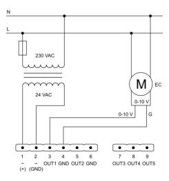
If you connect other devices to the same AC power source as the NL sensor, it is necessary to meet GND wiring of all analog inputs and outputs, as well as power wires.
